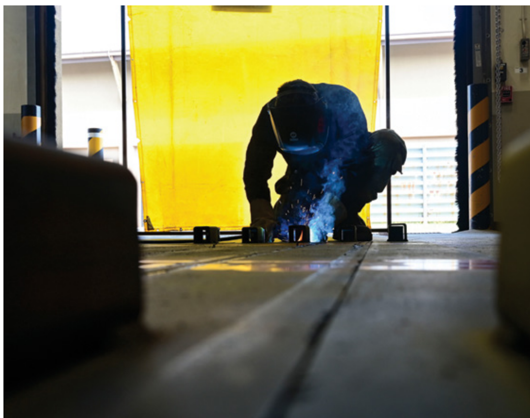
Airman 1st Class Dominic Varoz, 8th Maintenance Squadron aircraft metals technology journeyman, uses a Metal Inert Gas (MIG) welder to weld brackets onto custom built railroad track covers at Kunsan Air Base, Republic of Korea, June 18, 2025. The aircraft metal technology section developed the railroad track covers to prevent safety mishaps occurring from personal transportation device crashes on the tracks at the entrance to Kunsan. ▲
